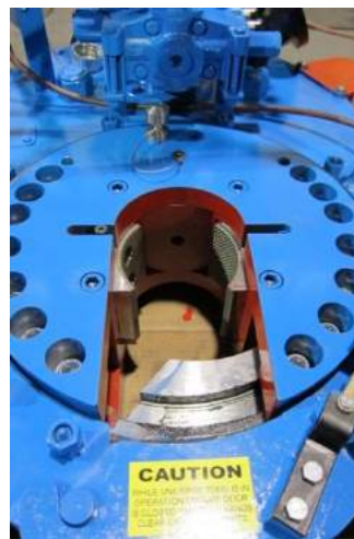
ROTATE RING GEAR TO BRING JAWS OUT OF SLOT
