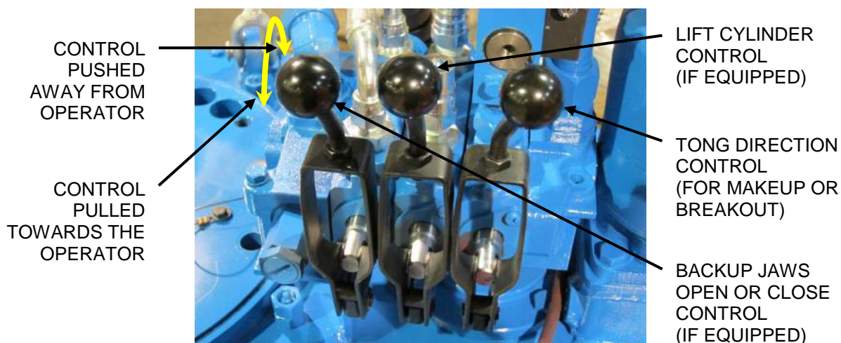
FIGURE 8.11: TONG VALVE BANK CONTROLS
