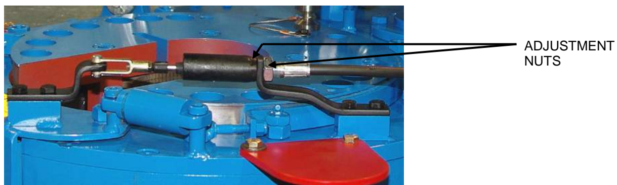
FIGURE 9.11: DOOR INTERFACE ADJUSTMENT
