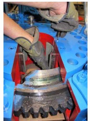
REMOVAL OF JAW WITH HELP OF SCREWDRIVER
