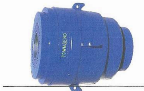
INCORRECT WAY TO STORE
